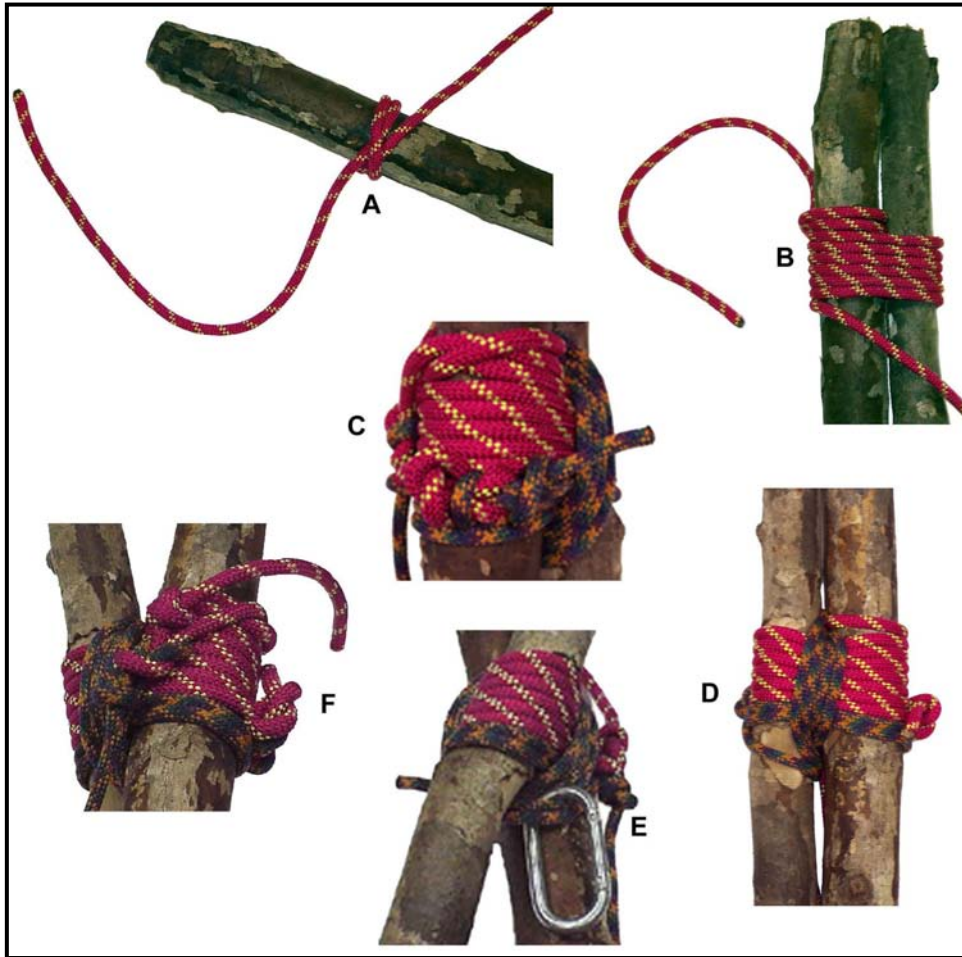
Figure 7-20. A-frame horizontal and vertical wraps.
